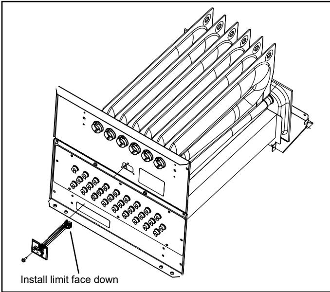
Figure 6. Primary Limit Location and Heat Exchanger
