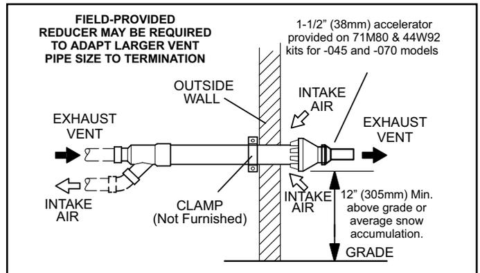
**Figure 37. Direct Vent Concentric Wall Termination
