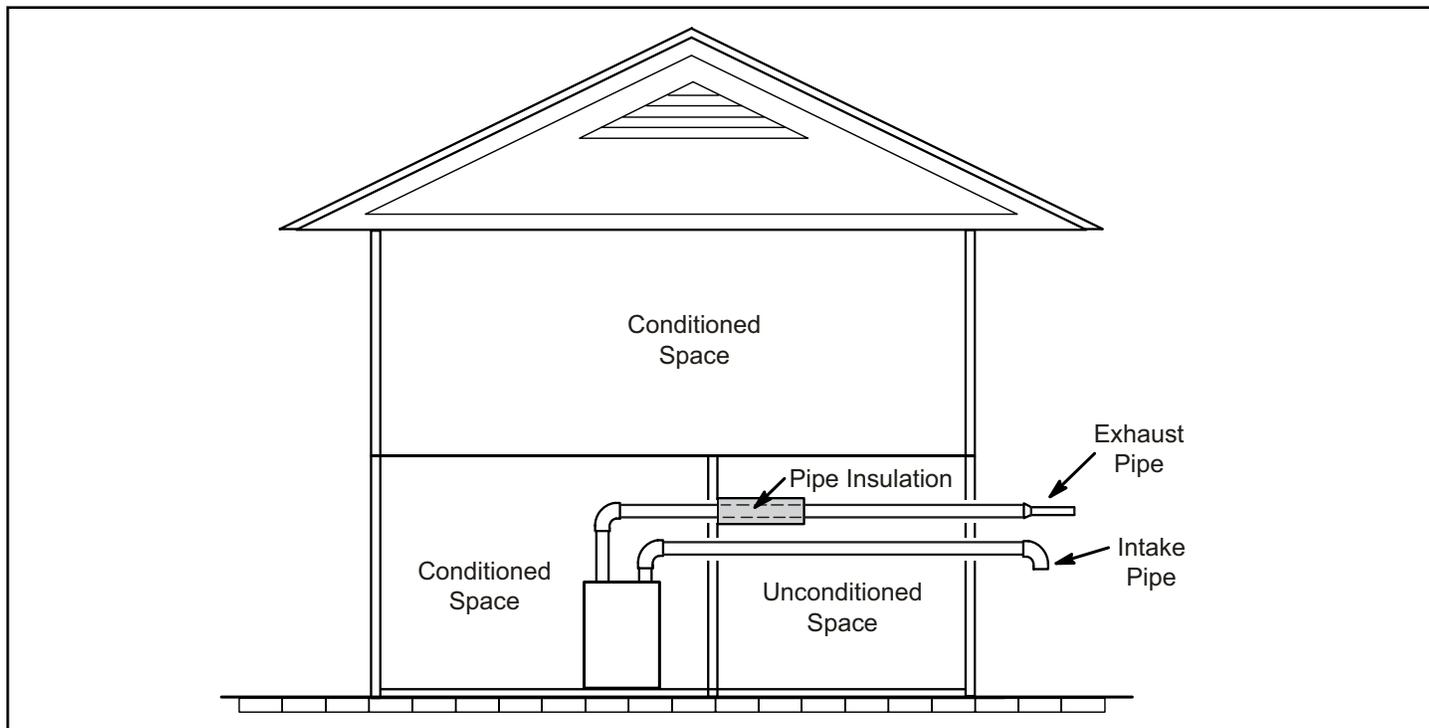
**Figure 29. Insulating Exhaust Pipe in an Unconditioned Space**
